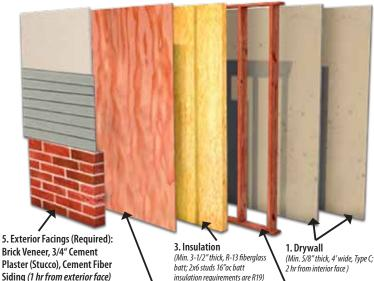
Siding (1 hr from exterior face) 4. FlamePRO Fire Retardant Treated Plywood
